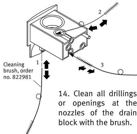
14. Clean all drillings or openings at the nozzles of the drain block with the brush.
