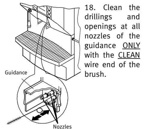
18. Clean the drillings and openings at all nozzles of the guidance ONLY with the CLEAN wire end of the brush.
