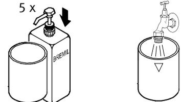
17. Insert the dispenser block, cover and coffee outlet into a cleaning bath once a time for 20 min.
