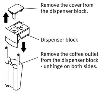
13. Clean all parts of the removed dispenser block individually under flowing warm water with the provided brush.
