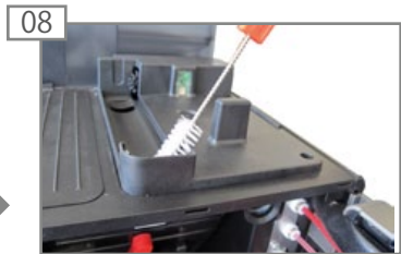
08 Clean the powder chute with a brush.
