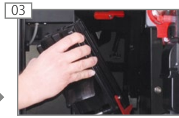
03 Remove the brewing unit.
