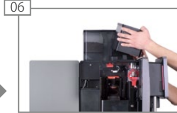
06 Lift the powder container up. Empty the powder container.
